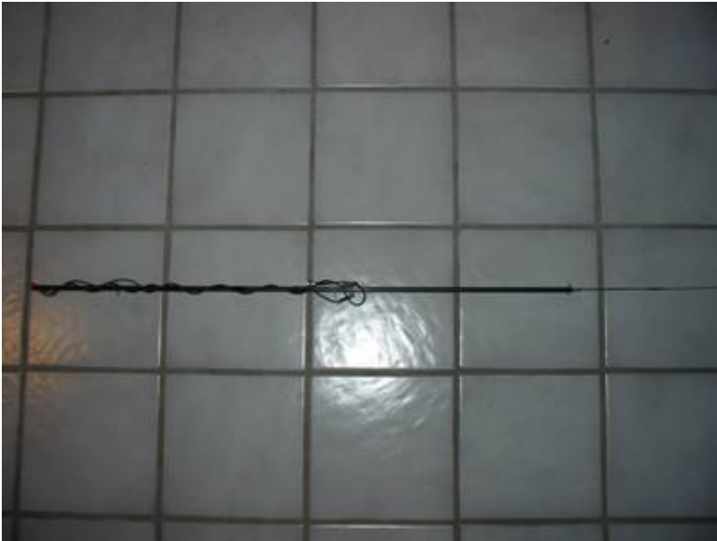
Fig. 5 Elements stored inside arrow shaft, coax wrapped around shaft. Vinyl sleeves remain in place always.
