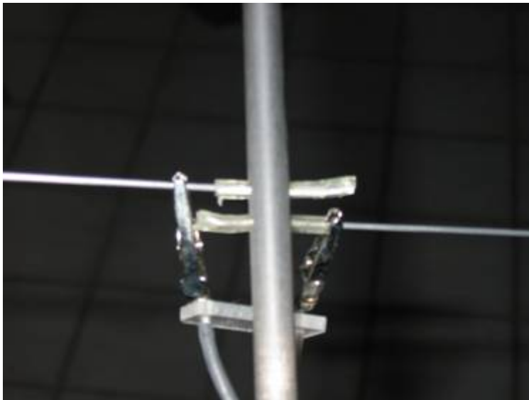
Fig. 4 Driven elements, alligator clip feed points, Plexiglas separator.
